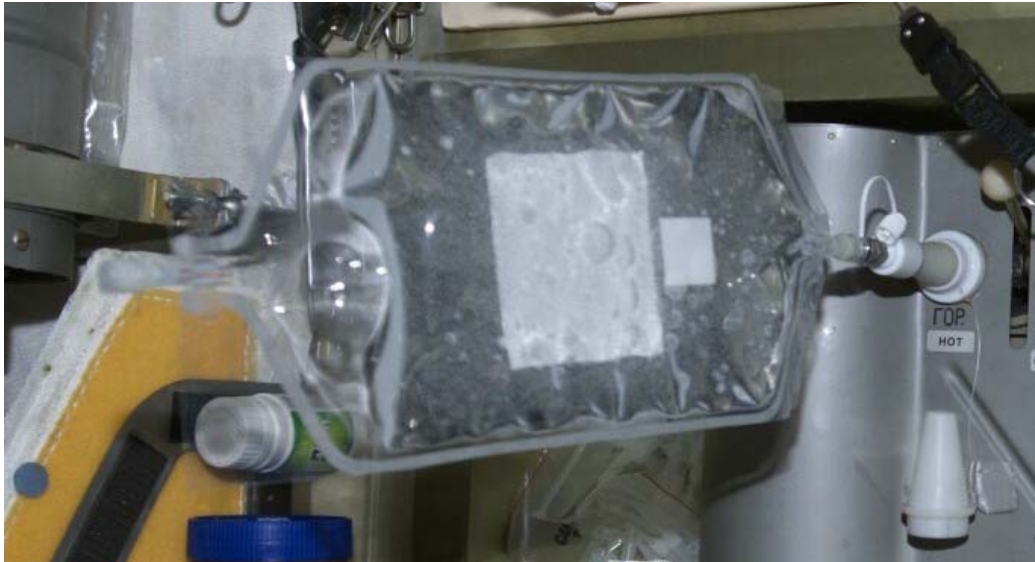
Figure 2. Photograph of typical air-water dispersion in a water sample collection bag on-board ISS.
