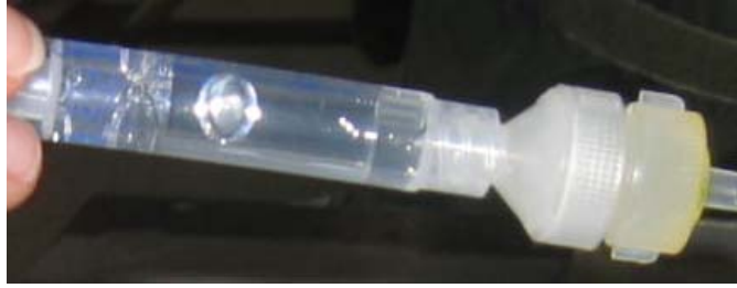
Figure 4. A 3.0-mL syringe after filling through glass wool cartridge in microgravity.
