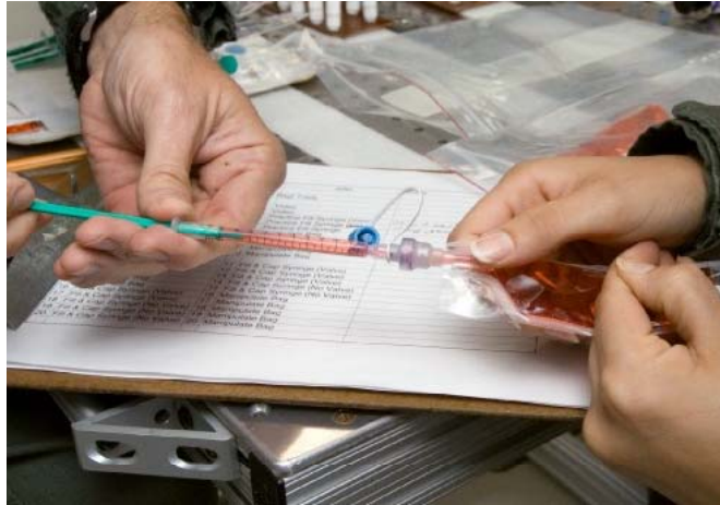
Figure 1. Filling a 1-mL syringe in-flight from a manually debubbled sample bag.
